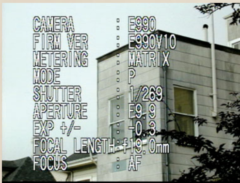
FIGURE 8.21 Most cameras will store a record of all the parameters you used for each shot. This data is stored with the file and can be read using special software.
